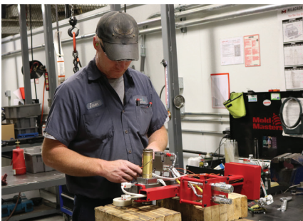
Clean water channels of mineral build-up.
