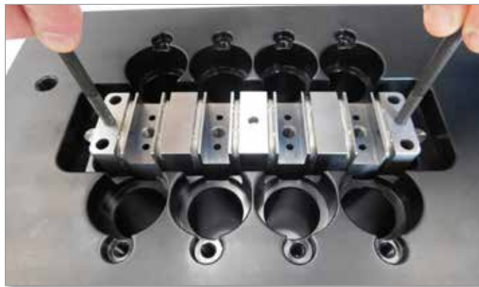
Figure 5-97 Install Melt-Cube manifold
