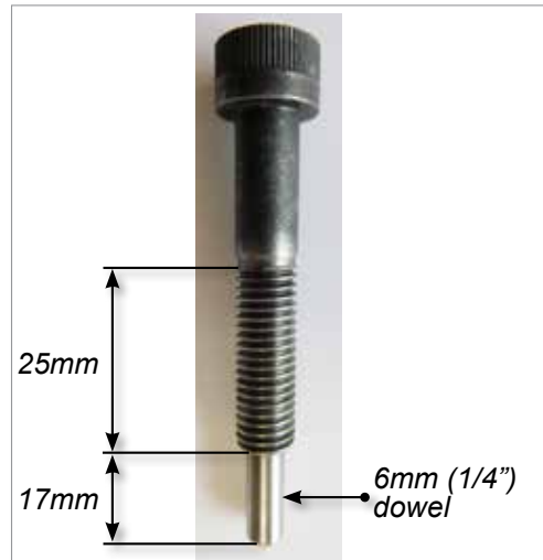
Figure 5-84 M10-1.5 jack bolt (SHCSM10X50-A)
