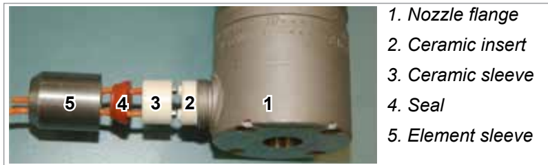
Figure 10-1 Nozzle terminal assembly
