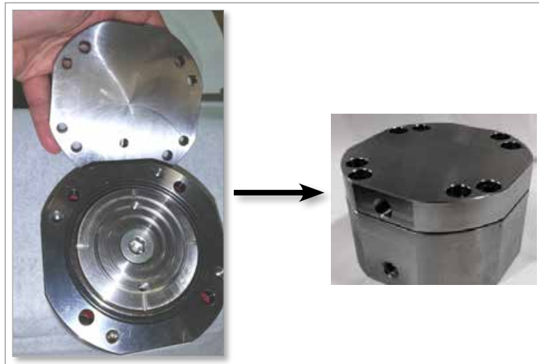
Figure 4-21 Assembled cylinder - note ports
