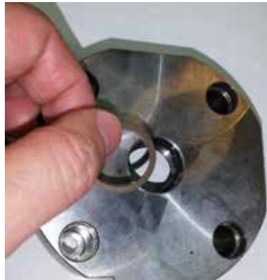
Figure 4-17 Install wiper seal
