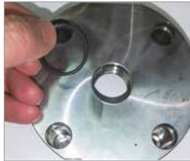
Figure 4-16 Install O-ring for wiper seal
