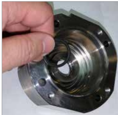
Figure 4-13 Install O-ring for rod seal
