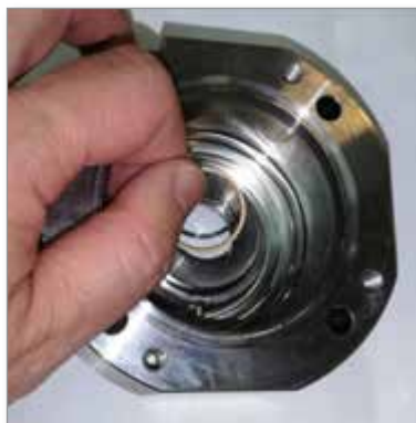
Figure 4-14 Install rod seal
