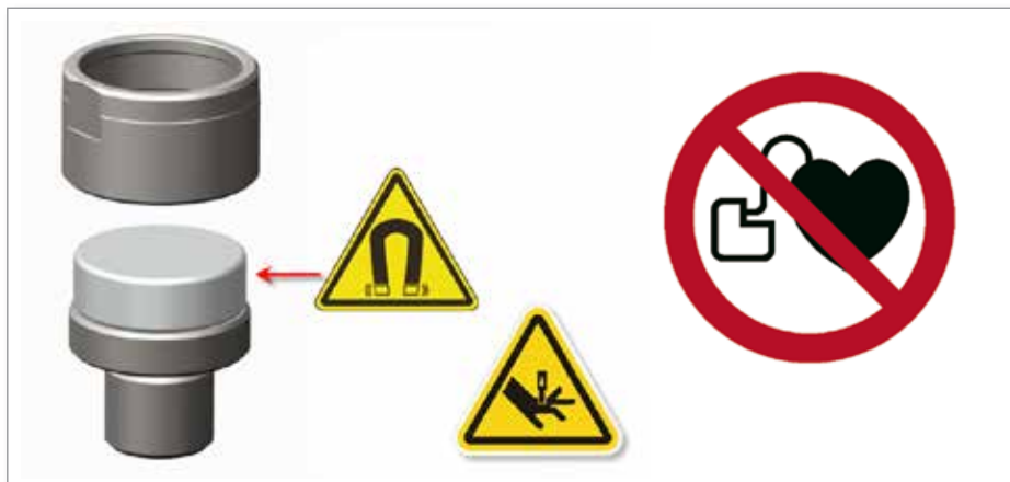
Figure 5-2 Mag-Pin safety hazards
